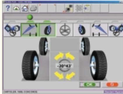
If the operator continues turning the wheel beyond this point, the machine knows that a toe-out-on turns measurement is desired and continues accordingly.
